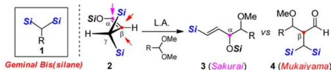
Scheme 1. General Structure of Geminal Bis(silane) (left); Sakurai vs Mukaiyama Adol Reaction of 3,3-Bis(silyl) Silyl Enol Ether with Acetal (right)
